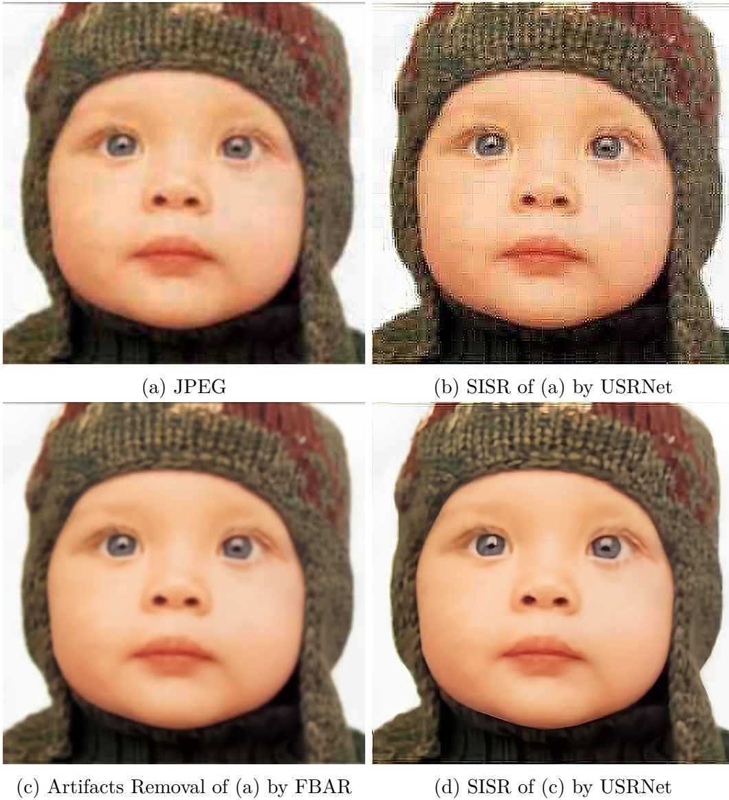
Figure 5.10.: Application of FBAR in image super-resolution. Our JPEG artifacts removal method can help to improve the performance of single image super-resolution.
