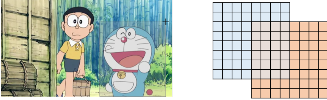
Figure 2.3.: An example of non-aligned double JPEG compression. Left: A common practical scenario when we want to crop out a region of interest from a JPEG image. If we save the region of interest also as JPEG, then a double JPEG compression occurs. Right: In this scenario, if the 8 \times 8 blocks of the newly saved image from the region of interest are not aligned with the blocks of the original JPEG image, then this is non-aligned double JPEG compression.
